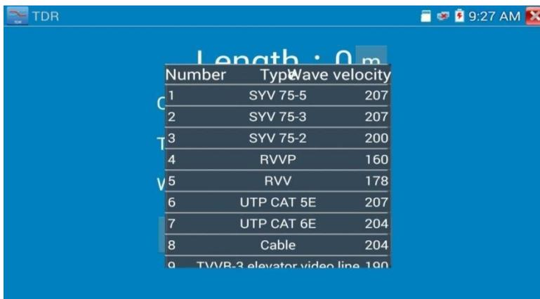
The screenshot shows a software interface with a blue background. At the top left, the text 'TDR' is visible. At the top right, there are system icons and the time '9:27 AM'. A large, semi-transparent text 'Length: 0 m' is overlaid on the screen. Below this, a table lists various cable types and their corresponding wave velocities. The table has three columns: 'Number', 'Type', and 'Wave velocity'. The rows are numbered 1 through 9.
